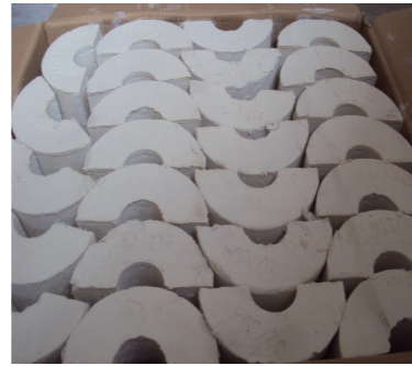
高性能矽酸鈣保溫材料 / High-performance calcium silicate thermal insulation material
